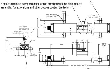
A standard 12 mm 5 pin micro connector is used. Straight mating cables can be ordered in a 6' length (949019L6), or 12' length (949019L12). If space is a consideration a right angle connector is also available, (949020L6 or 949020L12).
